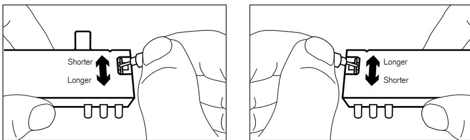
Using the screwdriver part of the adjustment tool, turn the rotaries in the directions shown to adjust the lag time.
